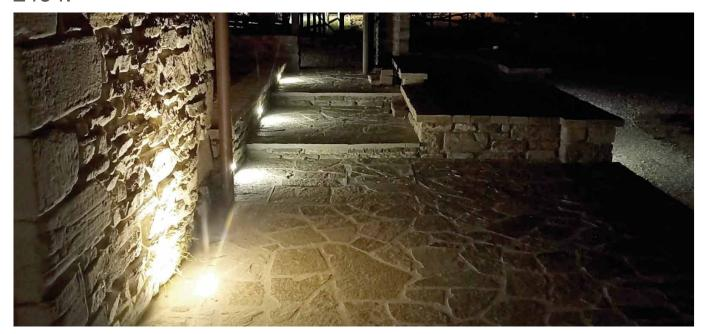
Flush-fitted in polished 304 stainless steel for accent, decoration, courtesy or step marker lighting. Anti-glare radial diffuser, can be installed indoors and outdoors. Mounting with formwork for brickwork.
